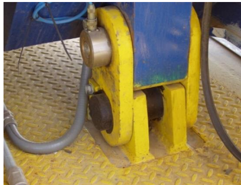
▲ Load control on a screed
