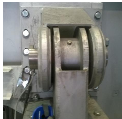
▲ Weighing tanks mounted on axes
